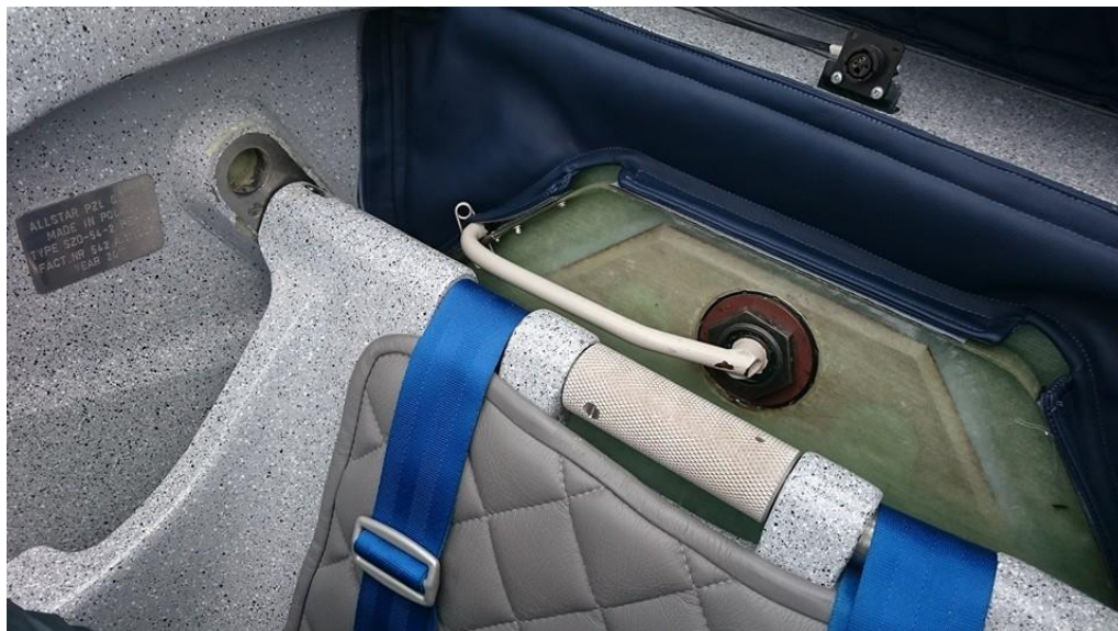
Rear backrest/seat pan adjustment: you turn the central cylindrical handle (between the shoulder straps) towards you to unlock the backrest (to retract the two ends of the rod), move it to the desired position and then screw the rod back into the cockpit sides.
