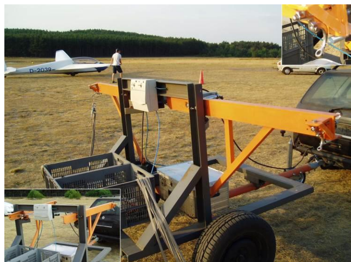
Cable tow-out, arms extended (inset: arms retracted + release mechanism)
